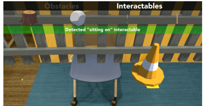
Figure 4. The Affordance Recommender detects predefined interactable classes (e.g. “chair” class corresponds to “sitting on” interactable).
